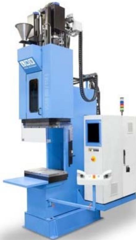
The process stability of the new TPE technology for two-component applications with EPDM was tested and optimized using a vertical machine by KRAIBURG TPE in collaboration with LWB Steinl.
