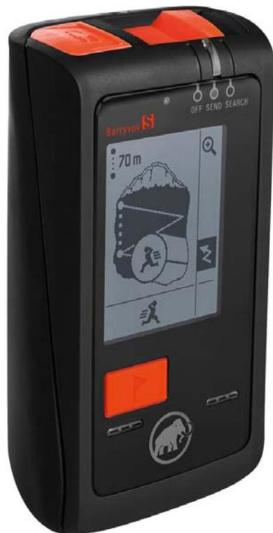
The Mammut® Barryvox® S locating device for winter sports enthusiasts, with an internal case seal and tactile casing elements providing highly secure grip qualities, made of mechanically robust and PA-compatible THERMOLAST® K from KRAIBURG TPE (photo: © 2018 Mammut Sports Group AG)
