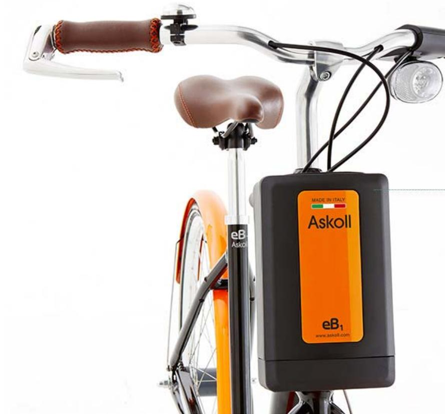
The battery of Askoll's power-assisted bicycles is mounted in a front compartment for convenient removal and recharge. Gaskets molded in THERMOLAST® K from KRAIBURG TPE provide a water-tight enclosure and anti-rattle performance in use. (Photo: © 2018 Askoll EVA)
